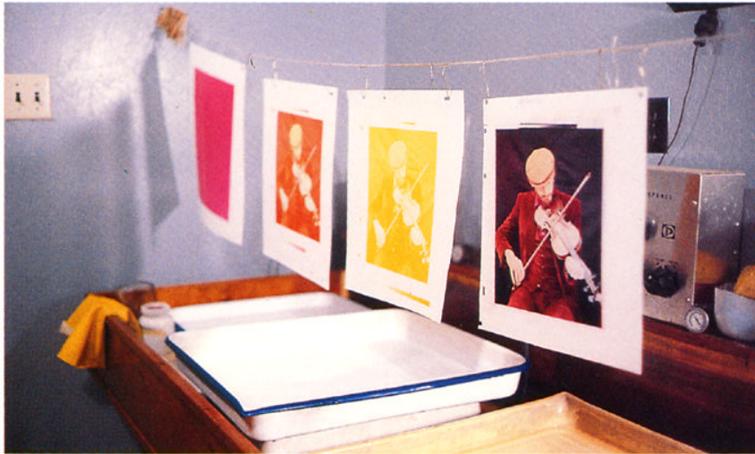
Assembly line: Separate pigment relief images (left) are assembled in precise register to make final Polaroid Permanent-Color print (extreme right).
