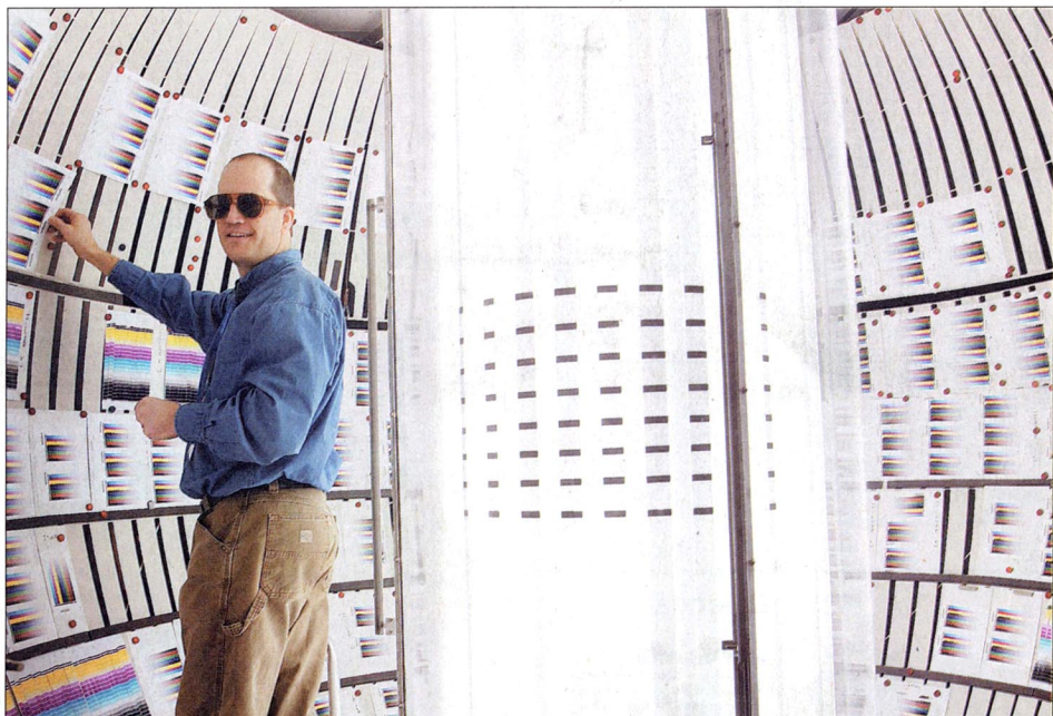
Keith Wright shows off a low-intensity fluorescent light fade chamber at Kodak's Building 69, where he's an image stability technician.
