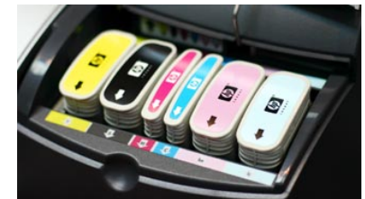
The HP Designjet 130 makes use of six HP Viverra high-stability dye-based photo inks.
