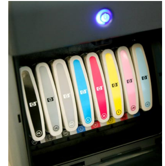
The HP Photosmart Pro 9180 is the first printer to use HP's newly developed, highly stable Vivera Pigment Inks. The eight ink cartridges include both Photo and Matte black inks along with a neutral Light Gray ink for enhanced black-and-white prints and also to reduce metamerism with both black-and-white and color images.
