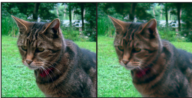
Figure 8. Image printed on System F, before (left) and after (right) 44 hours of exposure to high humidity. Very noticeable loss of sharpness is consistent with poor LQR response. Only minor change is seen in color as predicted by I^* results.
