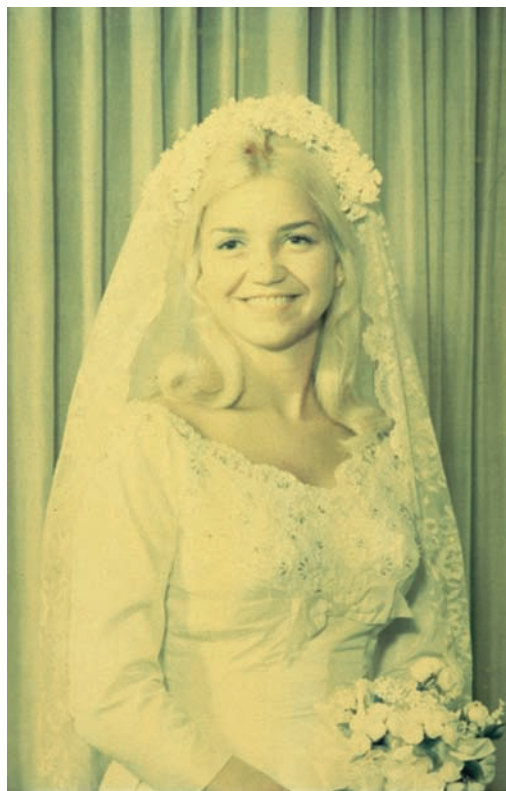
After only seven years of home display, this 1971 Kodak Ektacolor RC print suffered severe magenta dye fading and developed a yellowish stain.
