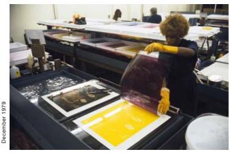
Kodak Dye Transfer prints are made by successively rolling three "matrix films" (which have been soaked in acidified cyan, magenta, and yellow dye solutions) into contact with the print surface. The matrix films have a gelatin layer that varies in thickness according to image density — the thicker the gelatin, the more dye it carries and transfers to the print.
