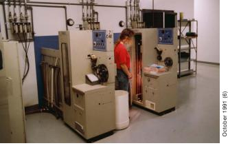
Of the thousands of rolls of film received by the lab each night, about 95 percent are Kodak, Fuji, and other C-41 compatible color negative films in the 35mm and, to a much lesser extent, 110 and 126 formats (Kodak Disc film has almost disappeared from the market). The film is spliced together in long rolls for processing in the machines shown above.
