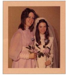
Kodak Ektacolor print after 120 days in accelerated dark fading/staining test.
