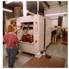
Rolls of exposed paper are processed in a six-strand Agfa RA-4 processor. After cutting, the prints and their negatives are put in customers' envelopes.
