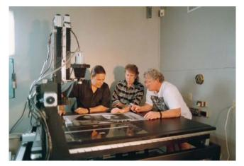
A high-resolution flatbed CCD scanner custom-built by Photometrics, Ltd. is used by Nash Editions to input images from color prints, paintings, and other art work. The scanner can accommodate originals of up to 4x4 feet.
