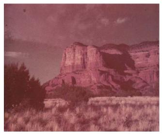
An Ektachrome 120 transparency shot in 1959 by Norman Rothschild and stored in the dark in New York City under normal room-temperature conditions since it was taken. The severe cyan and yellow dye loss is characteristic of the Kodak Process E-1, E-2, and E-3 Ektachrome films in use from 1946 until 1976.
