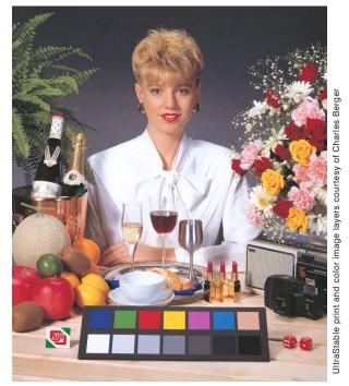
UltraStable Permanent Color print with an image composed of cyan, magenta, yellow, and black pigment layers. The print was made from a 6x7-cm transparency supplied by Fuji as an aid for setting up graphic arts color scanners.
