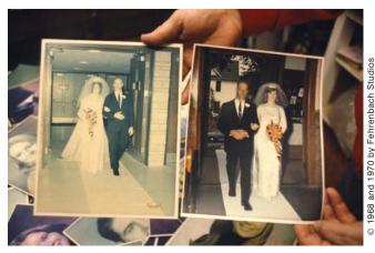
Displayed under similar lighting conditions in a home, the Ektacolor RC print on the left faded much more than the fiber-base Ektacolor Professional print on the right, even though the RC print had been displayed for a shorter period when this photograph was taken in 1981.
