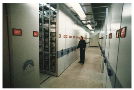
The color film storage vault in the Paramount Pictures Film and Tape Archive, located on the Paramount studio lot on Melrose Avenue in Hollywood, California. The color film vault, one of nine vaults in the high-security building, is kept at 40°F (4.4°C) and 25% RH. The multi-million-dollar facility went into operation in 1990. Shown here in the color film vault, which is equipped with movable shelving to conserve space, is Robert McCracken, a supervisor in Archive Operations.
