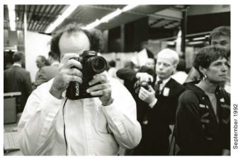
The Kodak Professional DCS 200 Digital Camera is built around a Nikon 35mm autofocus camera body. Instead of film, the camera uses a CCD (charge-coupled device) image sensor; the images are recorded on a small hard disk drive in the base of the camera. Introduced in 1992, the \$10,000 camera is shown here being demonstrated at the Photokina trade show in Germany.
