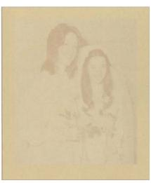
Kodak Ektacolor Plus print after light exposure in an accelerated test equivalent to 250 years of display. (The print was exposed to 21.5 klux glass-filtered fluorescent illumination for 2.7 years [75°F and 60% RH].)
