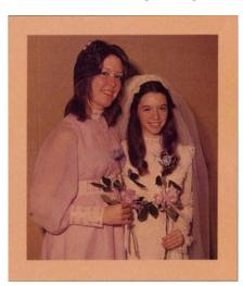
Kodak Ektacolor print after 240 days in accelerated dark fading/staining test.
