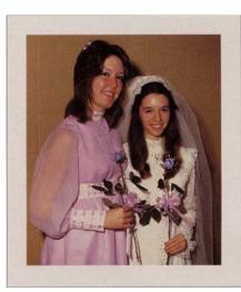
Fujicolor SFA3 print after 240 days in accelerated dark fading/staining test.
