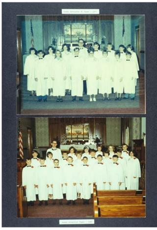
The upper print, made in 1971 with Ektacolor RC paper, faded much more than the lower print, made in 1968 with fiber-base Ektacolor Professional Paper, even though the fiber-base print had been displayed for 3 years longer than the RC print when this picture of the two choir photographs was taken in 1980. Both prints were framed under glass and had been on display next to each other in a church under similar lighting conditions.
