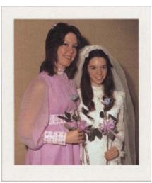
Polaroid Permanent-Color print after light exposure in an accelerated test equivalent to 575 years of display. Some magenta fading occurred, but the print remains in good condition. (The print was exposed to 21.5 klux fluorescent illumination for 6 years.)
