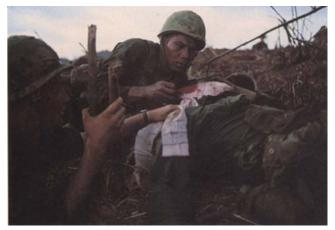
Kodak Dye Transfer fiber-base print after one year in the accelerated dark fading/staining test. The print showed almost no fading and suffered only slight staining. The one-year test period was twice as long as that used with the now-obsolete Ektachrome and Fujichrome papers below.
