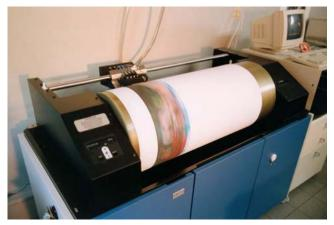
Iris ink jet printers lay down the cyan, magenta, yellow, and black images in a single pass with the print material attached to a rapidly rotating drum. The leading band of the image printed by the cyan ink jet, which slowly moves across the image from left to right, is clearly visible.
