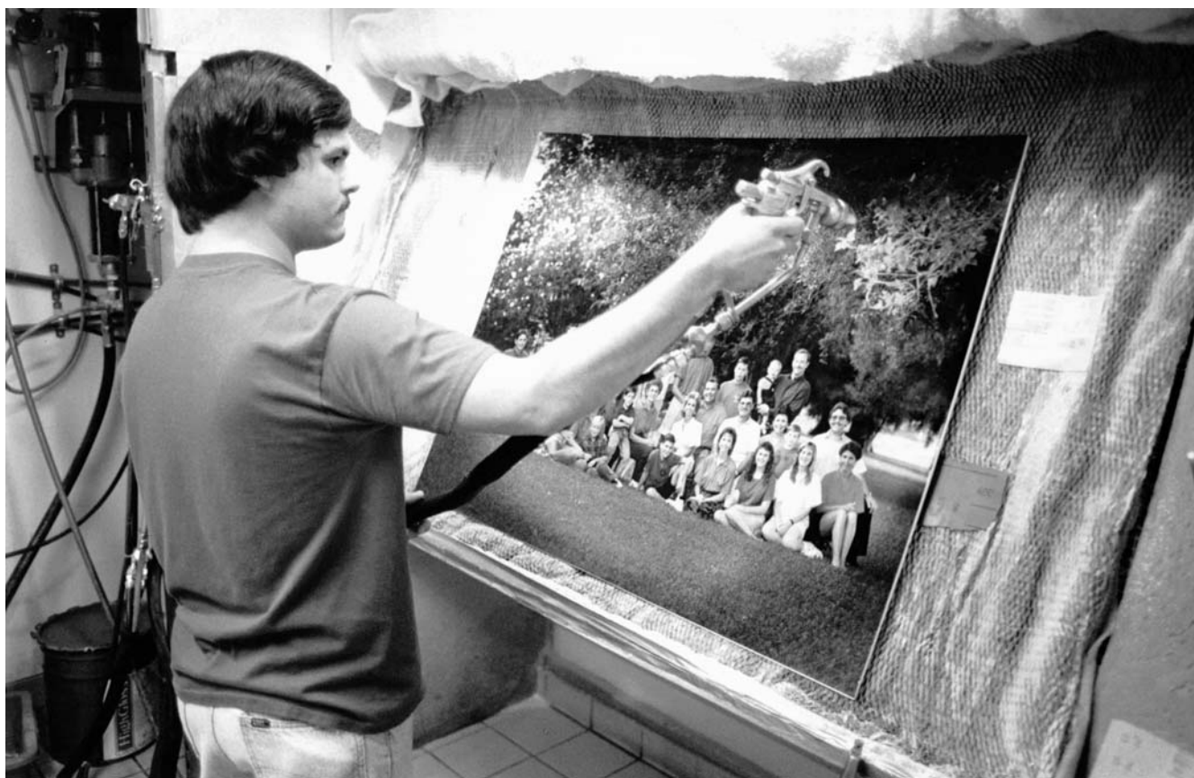
H&H Color Lab, located near Kansas City in Raytown, Missouri, is a leading Midwest lab serving professional portrait and wedding photographers. As is the case with most professional portrait labs, H&H's customers usually request lacquering on larger-size prints. Shown here is print sprayer Tom White lacquering a color print. H&H was the first professional portrait and wedding lab in the U.S. to switch from Kodak Ektacolor paper to Fujicolor paper. The change in color papers, which took place in 1991, was made because of the much better image stability of the Fuji product (see Chapter 8).
