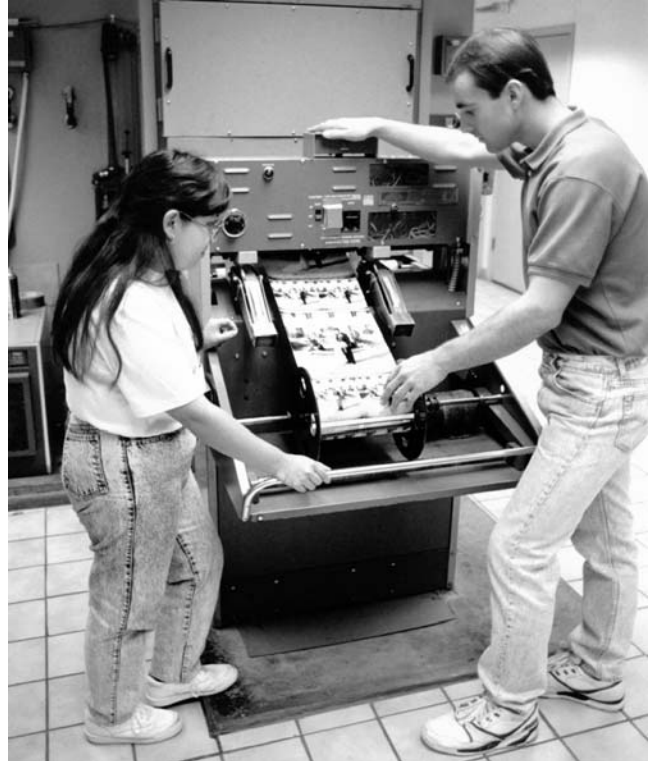
Printer inspector Sue Cadena and quality assurance manager Rob Newbanks checking Fujicolor prints coming off a Pako Leader Belt Processor Model 2140 which has been modified to run the RA-4 process. H&H uses Fuji-Hunt processing chemicals throughout the lab.
