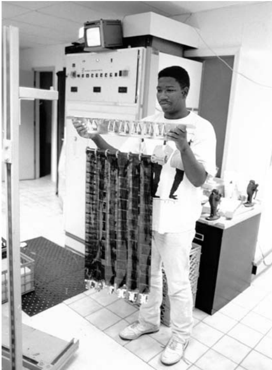
H&H film technician Darryl Owens with rolls of 220 Vericolor and Fujicolor color negative films that have been processed in a Sitte Tischer Divomat MX-24 dip-and-dunk processor. For protection against scratches, dust, and fingerprints, all film is sleeved immediately after processing (films remain sleeved during analyzing and proofing).
