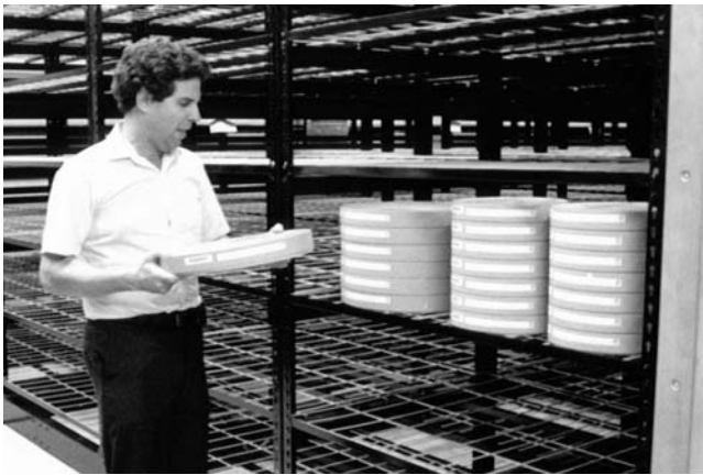
Prior to moving films into the new facility, Warner Bros. instituted a massive program to re-can all of its film in new bar-coded "vented" plastic film cans to prevent the "vinegar syndrome" — the accumulation of acetic acid vapors and other harmful acetate film-base deterioration by-products within the film cans. The building is equipped with a redundant activated charcoal air-filtration system to remove acetic acid vapors, peroxides, formaldehyde, and other potentially harmful substances from the air.
