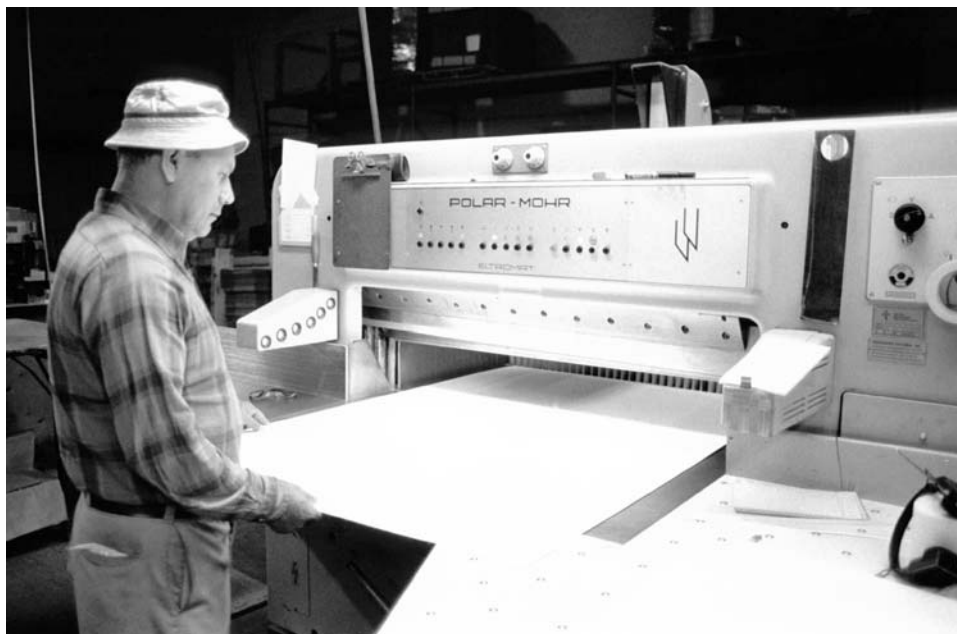
Mario Santiago of Crestwood Paper Company (New York/New Jersey) operates one of the company's two large computerized paper cutting machines. Most major paper distributors have at least one such machine to cut down large sheets and/or thick stacks of mount board and paper to customers' required sizes. (In October 1989, Crestwood merged with Andrews/Nelson/Whitehead to become ANW-Crestwood Paper Company.)
