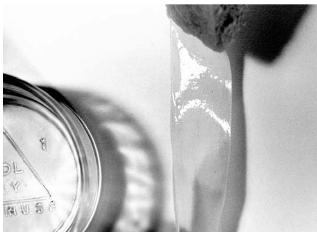
Overly moistened tape.
