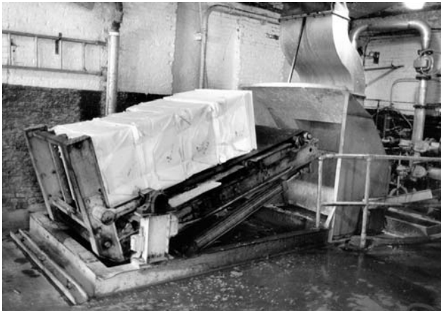
3. The bales are placed on a slowly moving conveyer belt which drops the pulp into the pulper.
