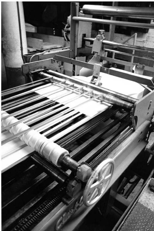
25. The 4-ply board is cut into sheets immediately as it leaves the dryers. Here the sheets are slightly larger than the standard size of 32 x 40 inches (by about 1/2 inch) to allow for trimming before packaging. The sheets land on a raised skid, which is gradually lowered to floor level by a hydraulic lift until the stack is full.
