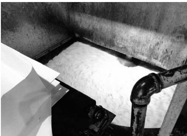
4. In this close-up, the pulper (approximately 10 feet in diameter) beats the pulp (furnish) into slurry. Most of the chemical ingredients, such as internal sizing agents, colorants, and alkaline buffers, are added to the pulp at this stage.
