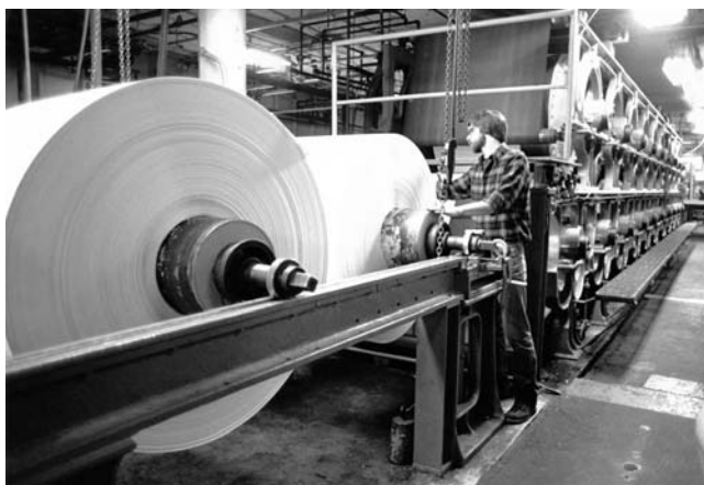
24. Pasting operator Mark Miller checks a roll of 4-ply board as it enters the dryers. Another recently pasted roll (left) will follow. Four-ply board takes about twice as long to dry as 2-ply.
