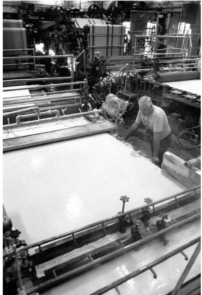
5. Machine tender Bob Hungerford looks over the wire (the wet end of the machine). A continuous belt made of fine fiber screen vibrates constantly as it moves forward so that the pulp fibers will mesh together and the water will drain away. It is during this stage that the grain direction is formed as the fibers line up in the direction of the flow.
