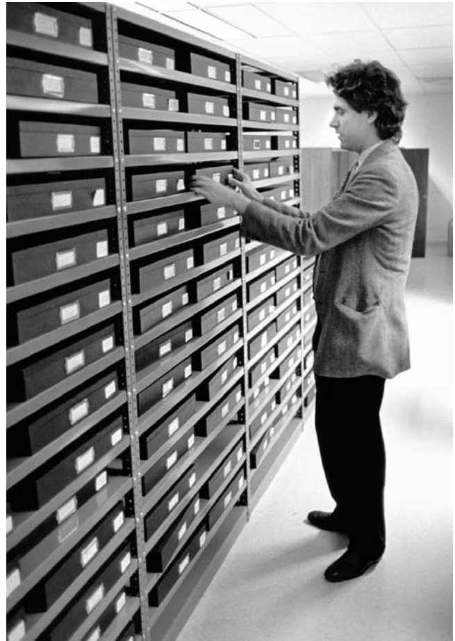
Print boxes are stored on steel shelves (coated with baked enamel) at the Museum of Modern Art in New York City. The shelves are open and no box rests on another; this provides ready access to the boxes and the prints. Here, Peter Galassi, now the director of the Department of Photography, removes a print box for study purposes. The photography collection is stored in an environmentally controlled room at 60°F (15.5°C) and 40% RH.
