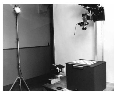
This camera set-up was devised by Daniel Jones for producing index slides. Slides in pages are lighted from below to illuminate the images, and from above so that serial numbers, dates, and caption information are visible. Kodachrome 40, a tungsten-balanced film, was chosen for the project because of its sharp, fine-grain images.
