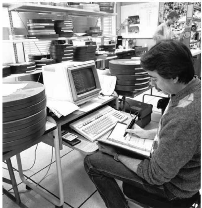
A computer-based catalog system tracks the films in the Archives. Operator Dennis Waugh inputs film titles and other data manually at a Hewlett-Packard computer terminal and uses a lightpen to read data from standardized preprinted bar codes. The bar-code labels are then affixed to the film cans.
