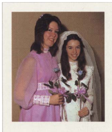
Polaroid Permanent-Color print after 6 years in an accelerated dark fading/staining test. No fading or staining of the image or polyester base material could be observed. (The accelerated test was conducted at 144°F [62°C] and 45% RH.)
