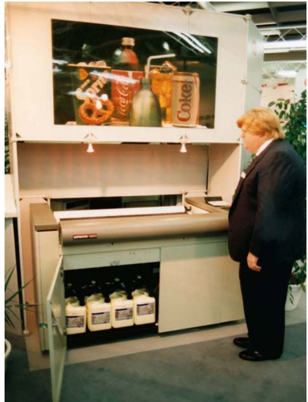
Xerox/Versatec color printer in a system supplied by Onyx Graphics (note containers of liquid toners in base).
