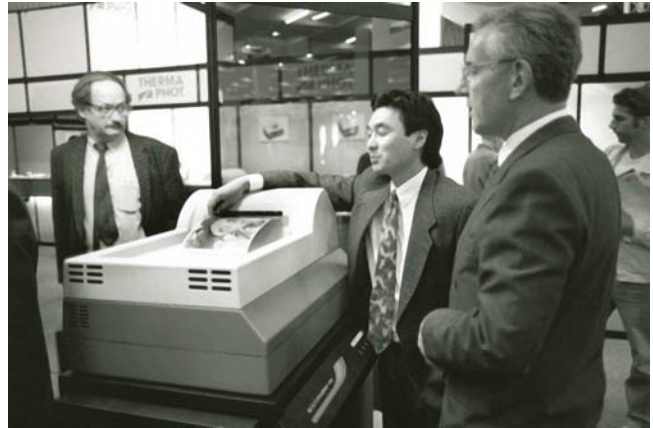
Metrum FotoPrint digital color printers produce 300 dpi “continuous-tone” prints with traditional RA-4 color papers.
