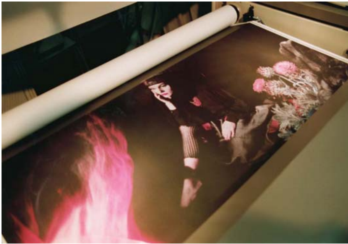
A large-format print emerging from a Xerox/Versatec liquid-toner electrostatic color printer. Used in the Cactus and Onyx Graphics digital printing systems, the Versatec units produce low-cost color prints in sizes up to 54 inches wide and 15 feet or more in length.
