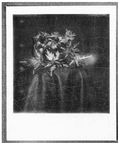
A Polaroid SX-70 color print made in 1973 that has developed internal image-receiving layer cracks. Early SX-70 prints (1972–76) are frequently found to have developed such cracks, especially if they have been stored in very dry conditions.
