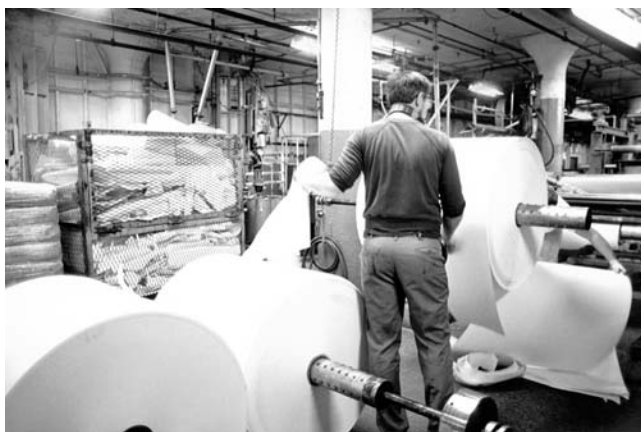
15. Pasting operator Kurt Bodendorf removes several outside layers before the rolls are hoisted onto the pasting machine.
