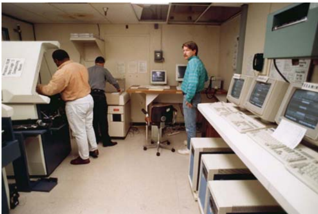
Fully composed digital pages with photographs in place are output to separation film on Linotronic and Autologic imagesetters. The films are used to make flexographic printing plates for the newspaper's high-speed presses.
