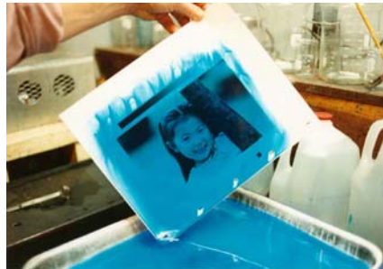
Unhardened pigmented gelatin is removed in a warm-water bath.
