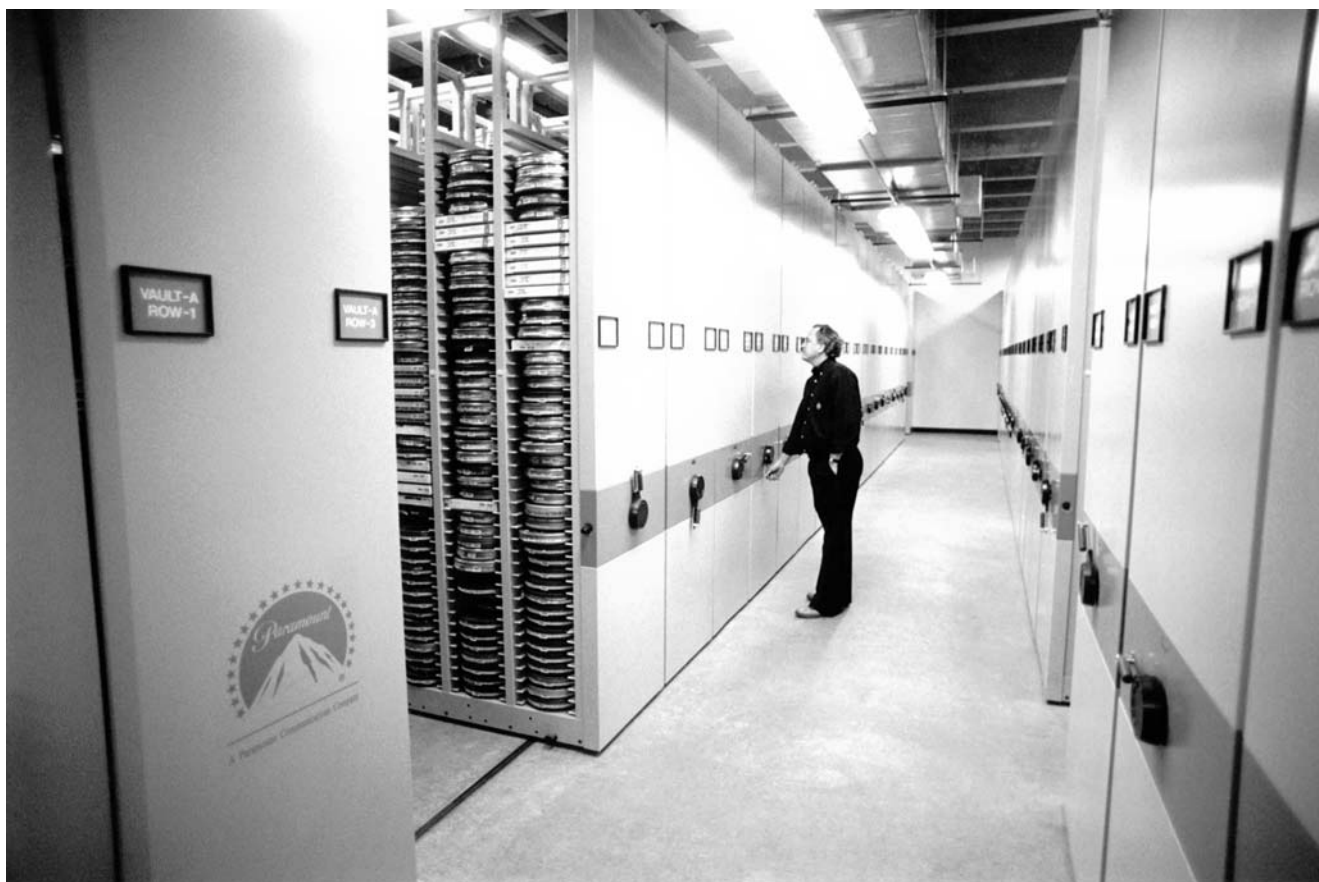
The color film storage vault in the Paramount Pictures Film and Tape Archive, located on the Paramount studio lot on Melrose Avenue in Hollywood, California. The color film vault, one of nine vaults in the high-security building, is maintained at 40°F (4.4°C) and 25% RH. The Paramount archive, which was Hollywood’s first adequate preservation facility for color motion pictures, went into operation in June 1990. Shown here working in the color film vault, which is equipped with movable shelving to conserve space, is Robert McCracken, a supervisor in Archive Operations. McCracken and Bill Weber, director of Operations Resources at Paramount, manage the operation of the multi-million dollar, 40,000-square-foot facility. At the time this book went to press in 1992, Warner Bros. was the only other Hollywood studio to have adequate cold storage facilities for its motion picture library (the new Warner Bros. film archive is described later in this chapter).
