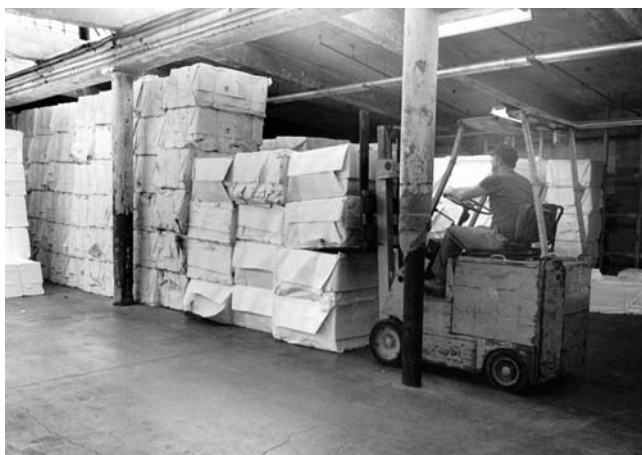
2. Dry sheets of 100% cotton linters pulp are stored in large bales at the mill, ready for making paper and museum board. Pulp operator Joe Stebbins is separating bales with a forklift truck to move them to the pulper.
