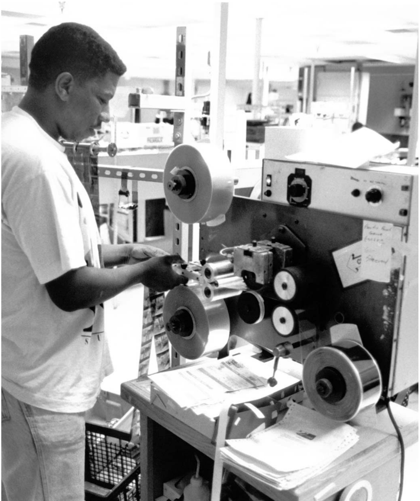
A Phototech hot-seal plastic sleeving machine in operation at H&H Color Lab under the watchful eye of Darrell Owens, a film processing technician. H&H, a leading professional portrait and wedding lab located near Kansas City in Raytown, Missouri, processes and proofs up to 2,000 rolls of color negative film a day (mostly in the 120/220 format). Sleeving is done immediately after processing to protect the film from dust and scratches. The film is video analyzed, proofed, and shipped to customers without ever removing the film from the sleeves.
