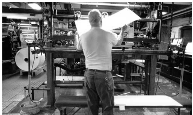
12. At the start of a new roll, the machine tender examines a sample of the 1-ply board before it is sent to the laboratory for specification tests (caliper or thickness, basis weight, color, consistency, strength, etc.). Requiring the attention of three separate shifts of workers, the machines run 24 hours a day, 7 days a week producing museum board and numerous other fine papers. The finished roll of 1-ply museum board is pictured on the left.
