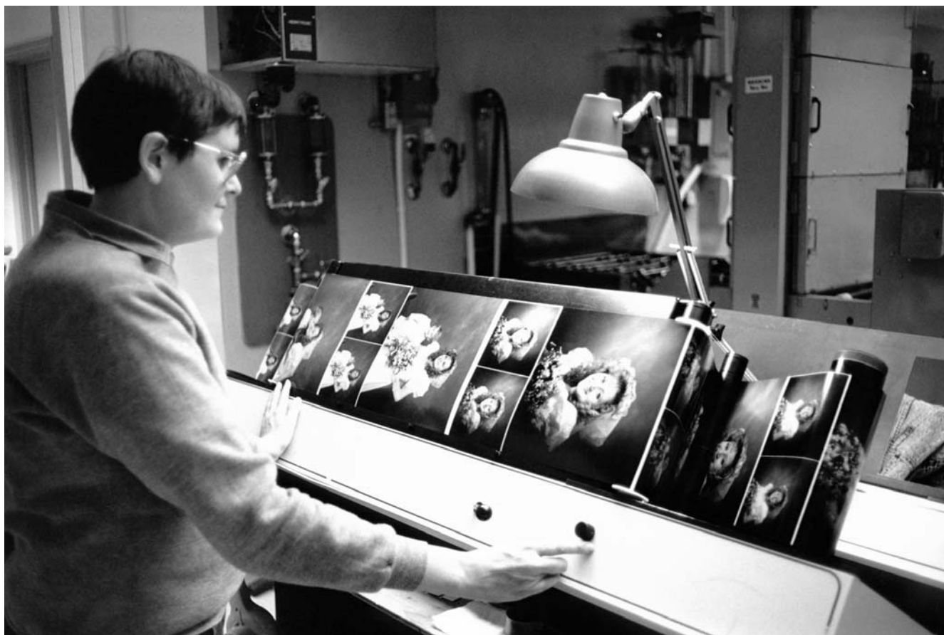
Wedding portraits printed on Fujicolor Professional Paper Super FA Type P being inspected at H&H Color Lab by printing department supervisor Steve Tuggle. H&H, a leading professional portrait and wedding lab located near Kansas City in Raytown, Missouri, switched from Ektacolor Portra paper to Fujicolor paper in 1990 because of the superior light fading stability of the Fuji product. The change in color paper was made after a poll mailed to more than 700 H&H customers showed that the great majority wanted their wedding photographs and portraits printed on the longest-lasting color paper available, even if that meant changing from Kodak to Fuji as the paper supplier (see Chapter 8).
