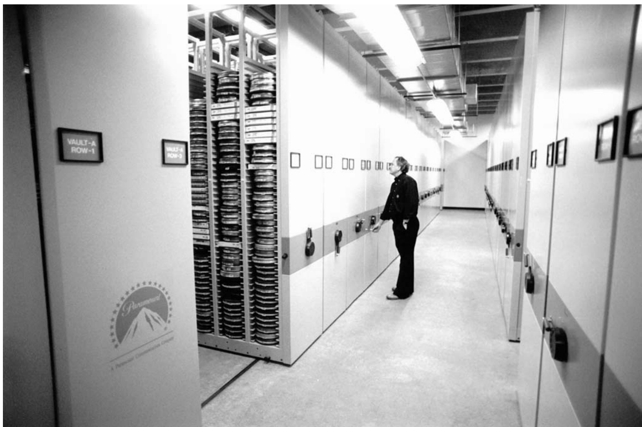
The color film storage vault in the Paramount Pictures Film and Tape Archive, located on the Paramount studio lot on Melrose Avenue in Hollywood, California. The color film vault, one of nine vaults in the high-security building, is maintained at 40°F (4.4°C) and 25% RH. The multi-million dollar facility went into operation in 1990. Shown here in the color film vault, which is equipped with movable shelving to conserve space, is Robert McCracken, a supervisor in Archive Operations.
