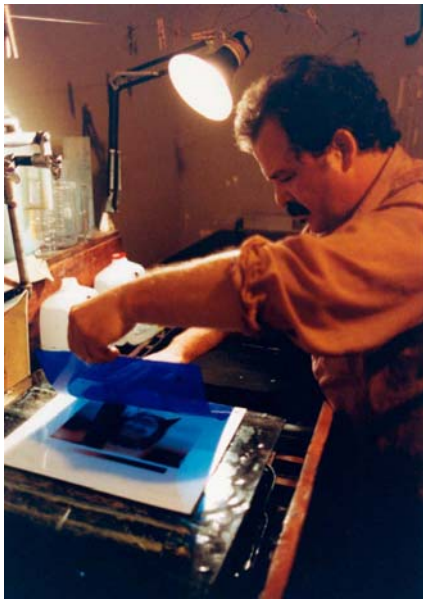
After exposure with separation negatives, the cyan, magenta, yellow, and black pigment layers are applied one at a time to a polyester or paper support.
