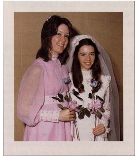
Fujicolor SFA3 color print after the equivalent of 50 years of display.
