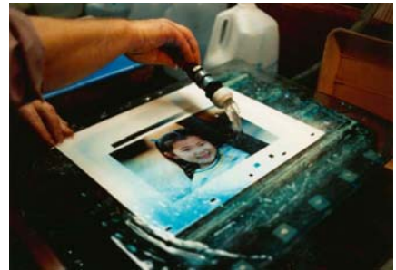
With all four image layers applied, the finished print is rinsed with water.
