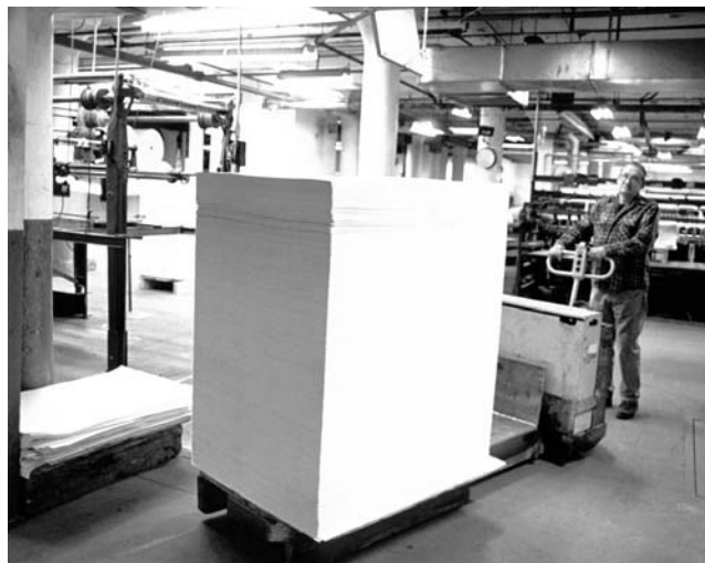
27. Forklift operator Francis Hansen takes the museum board to be weighed. This stack weighs about 1,250 pounds. Afterward, the board will be trimmed to 32 x 40 inches, sorted by hand to remove sheets with surface defects, arranged into groups of 10 or 25 sheets, wrapped in water-resistant paper, and packaged in corrugated cartons for storage in the warehouse before it is sent to distributors.
