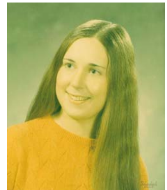
1969 Ektacolor RC print after 13 years of display.
