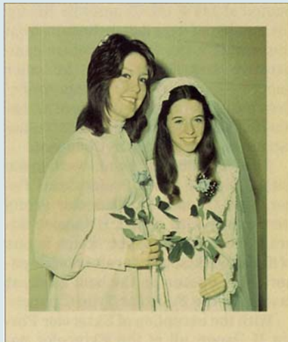
Kodak Ektacolor print after the equivalent of 50 years of display.
