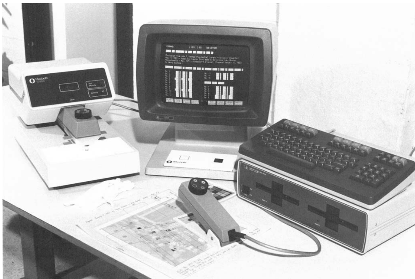
Density measurements of a color print are read with a Macbeth TR924 densitometer (left). Data are transmitted by the densitometer to this author's microcomputer (center) and recorded on disk (right). The computer is programmed to analyze data in terms of specified densitometric limits of change.
