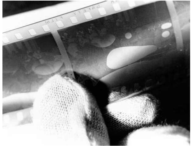
With the negative removed from its sleeve, damage in the form of irregular gloss on the emulsion surface is clearly visible. The sticking occurred after about 5 years of storage under normal conditions in this author's house in Grinnell, Iowa.
