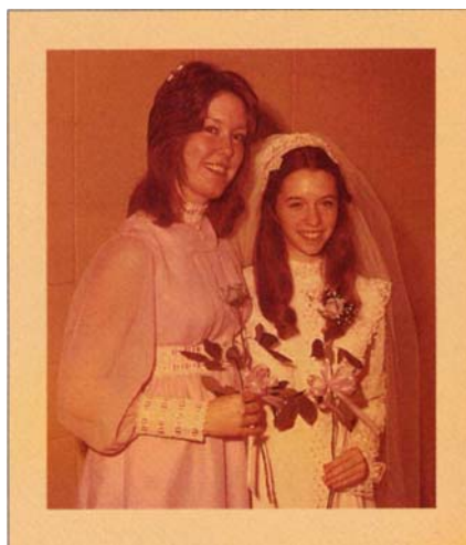
Kodak Ektacolor 74 RC print after 240 days in accelerated dark fading/dark staining test.
