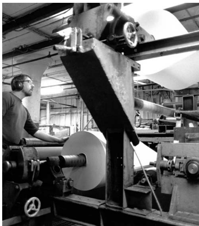
16. To make 2-ply board, one roll of 1-ply board is suspended above another roll. They unroll together at a rate of about 450 feet per minute. Bodendorf supervises the operation as the lower roll passes through the pasting applicator (lower right).
