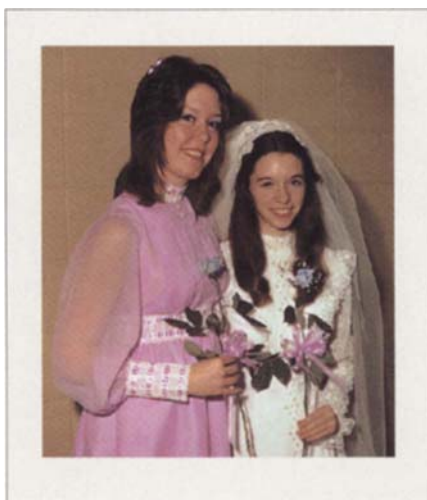
Polaroid Permanent-Color print after light exposure in an accelerated test equivalent to 575 years of display. Some magenta fading occurred, but the print remains in good condition. (The print was exposed to 21.5 klux fluorescent illumination for 6 years.)
