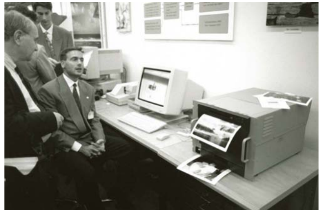
Kodak Ektatherm XL 7700-series digital printers, one of which is shown here at the Photokina trade show in Germany in 1992, produce “continuous-tone” 200 dpi “photorealistic” thermal dye-transfer color prints from digital image files. Thermal dye-transfer (dye-sublimation) printers supplied by Kodak and other manufacturers cost between $10,000 and $25,000.
