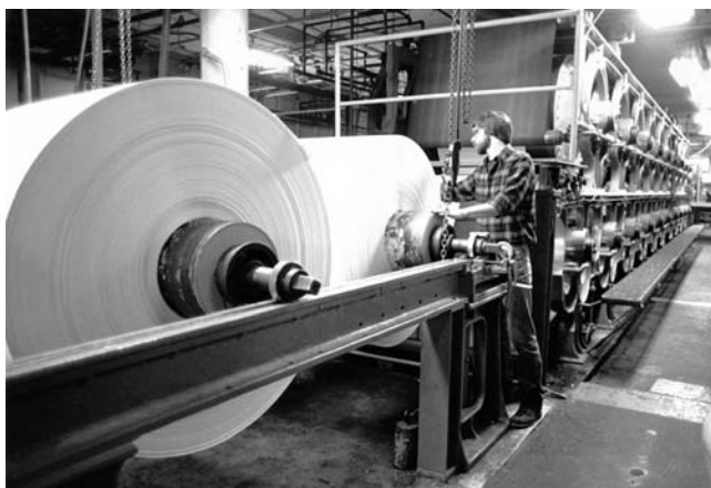
24. Pasting operator Mark Miller checks a roll of 4-ply board as it enters the dryers. Another recently pasted roll (left) will follow. Four-ply board takes about twice as long to dry as 2-ply.
