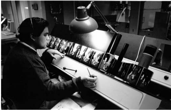
Steve Valenzuela, print spotter/inspector at H&H, checking prints prior to cutting and packaging. All prints from 120/220 negatives are routinely dust-spotted (retouched to remove small dust spots).
