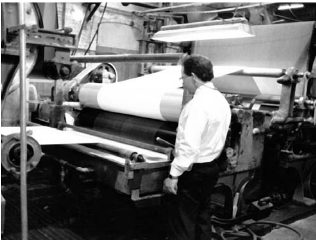
9. Marketing and sales manager Thomas Richards looks over the paper as it comes out of the first set of dryers and enters a bath containing surface sizing chemicals. The paper then enters a second set of dryers (right).
