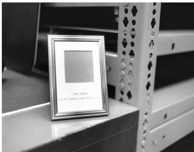
An Agfa-Gevaert colloidal silver test slide, matted and in a small metal frame (without glass), in the photograph storage vault at the Art Institute of Chicago.
