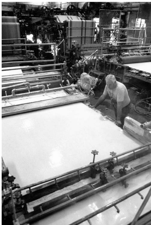
5. Machine tender Bob Hungerford looks over the wire (the wet end of the machine). A continuous belt made of fine fiber screen vibrates constantly as it moves forward so that the pulp fibers will mesh together and the water will drain away. It is during this stage that the grain direction is formed as the fibers line up in the direction of the flow.
