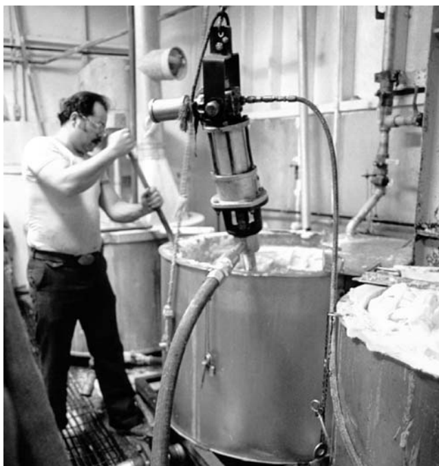
17. Carlos Cruz mixes the sacks of dry starch-based adhesive with water to produce the proper consistency before the adhesive enters the pasting applicator. Starch paste is preferable to animal glues or synthetic adhesives for laminating high-quality boards because it is more stable chemically, does not discolor, and does not contain residual chemicals and acids, which break down the paper fibers.
