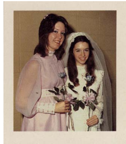
Kodak Ektacolor print after the equivalent of 10 years of display.
