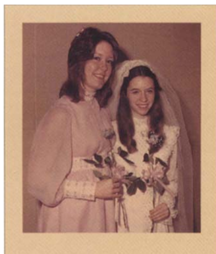
Kodak Ektacolor Plus print after one year in an accelerated dark fading/staining test. Note the severe, overall yellowish staining of the image. (The accelerated test was conducted at 144°F [62°C] and 45% RH.)
