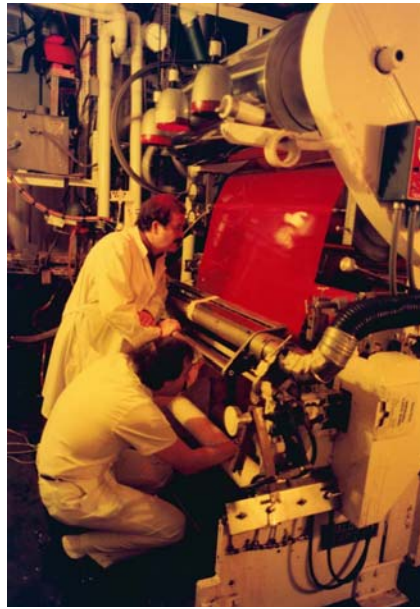
Coating the magenta emulsion on a transparent polyester carrier sheet.
