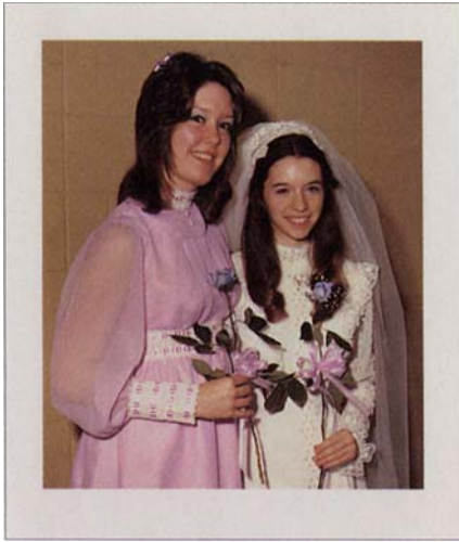
Fujicolor SFA3 color print after the equivalent of 15 years of display.
