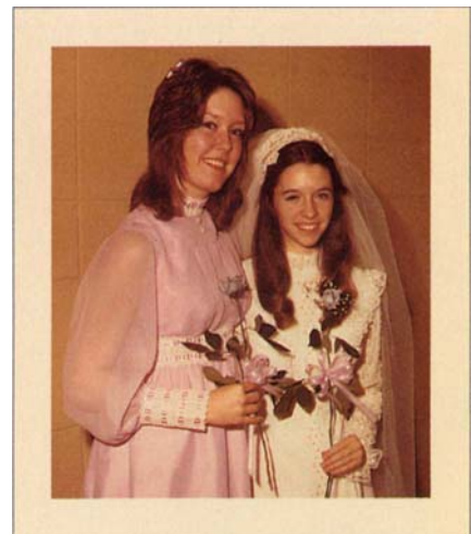
Kodak Ektacolor 74 RC print after 60 days in accelerated dark fading/dark staining test.
