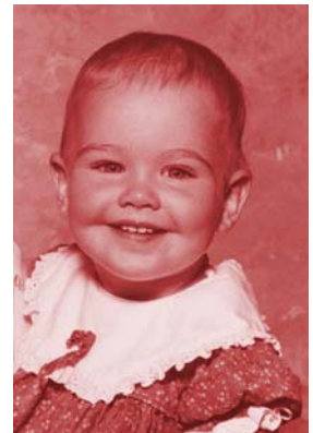
1980 Agfacolor print kept in the dark (note cyan fade).
