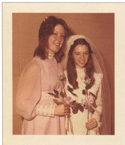
Kodak Ektacolor 74 RC print after 120 days in accelerated dark fading/dark staining test.
