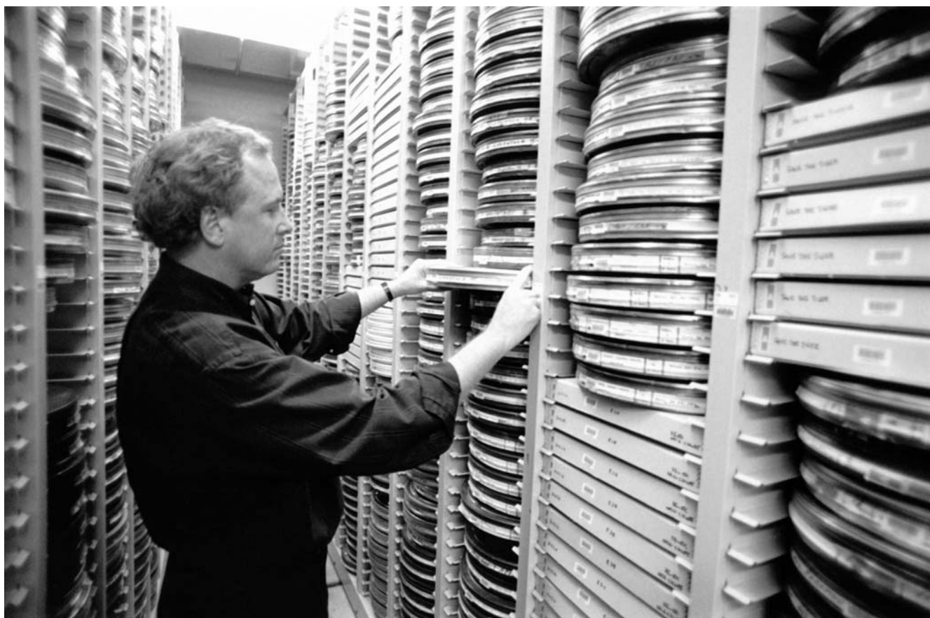
Specially designed shelves hold each roll of film in a separate slot, which simplifies locating a specific roll and avoids the handling difficulties that can occur when rolls are stacked. Paramount has inaugurated a program to repackage films in special, alkaline-buffered cardboard boxes to prevent the gradual accumulation of acetic acid vapors that can occur in regular film cans as a result of acetate film-base decomposition (the “vinegar syndrome”). If acetic acid vapors are not vented or otherwise removed, both dye fading and film-base deterioration can be accelerated. The air in the vault is filtered to remove acid vapors and other contaminants. McCracken is shown here pulling a can containing a roll of the original camera negative from Francis Ford Coppola’s 1974 classic, The Godfather, Part II . The film, which won six Academy Awards, including Best Picture, Best Director, and Best Screenplay, starred Robert DeNiro, Robert Duvall, Diane Keaton, and Al Pacino.
