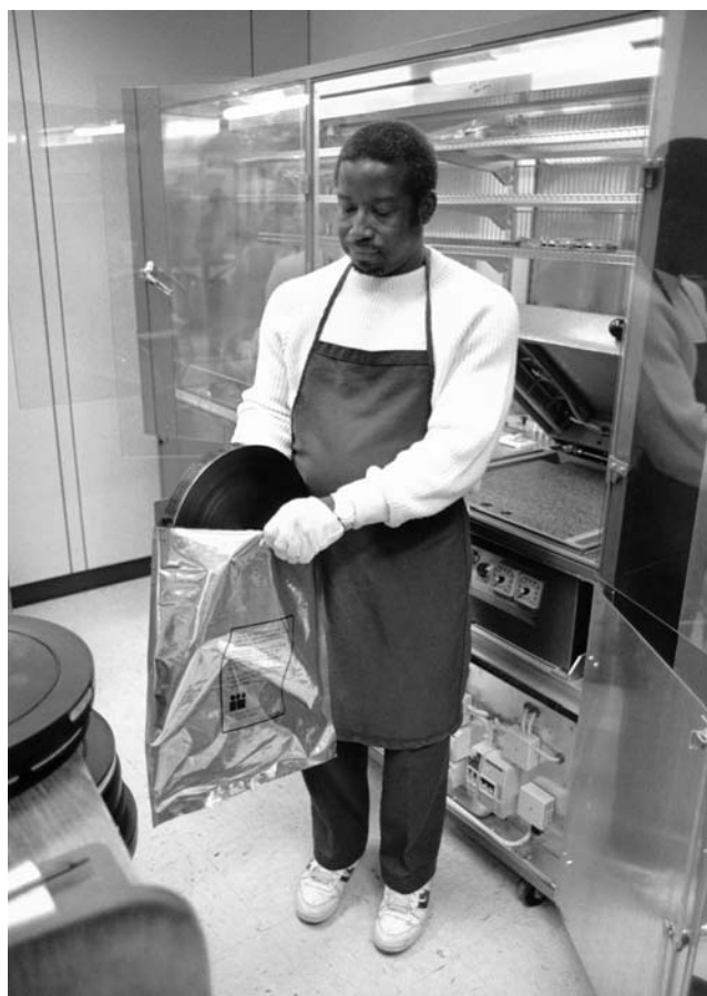
A Swedish FICA film-conditioning and vacuum-sealing machine at the Motion Picture, Broadcasting, and Recorded Sound Division of the Library of Congress in Washington, D.C. Film technician David Lee Reese prepares to vacuum-seal a vapor-proof bag containing a roll of film that has been equilibrated to a low moisture content in the machine. The system is no longer used by the Library.
