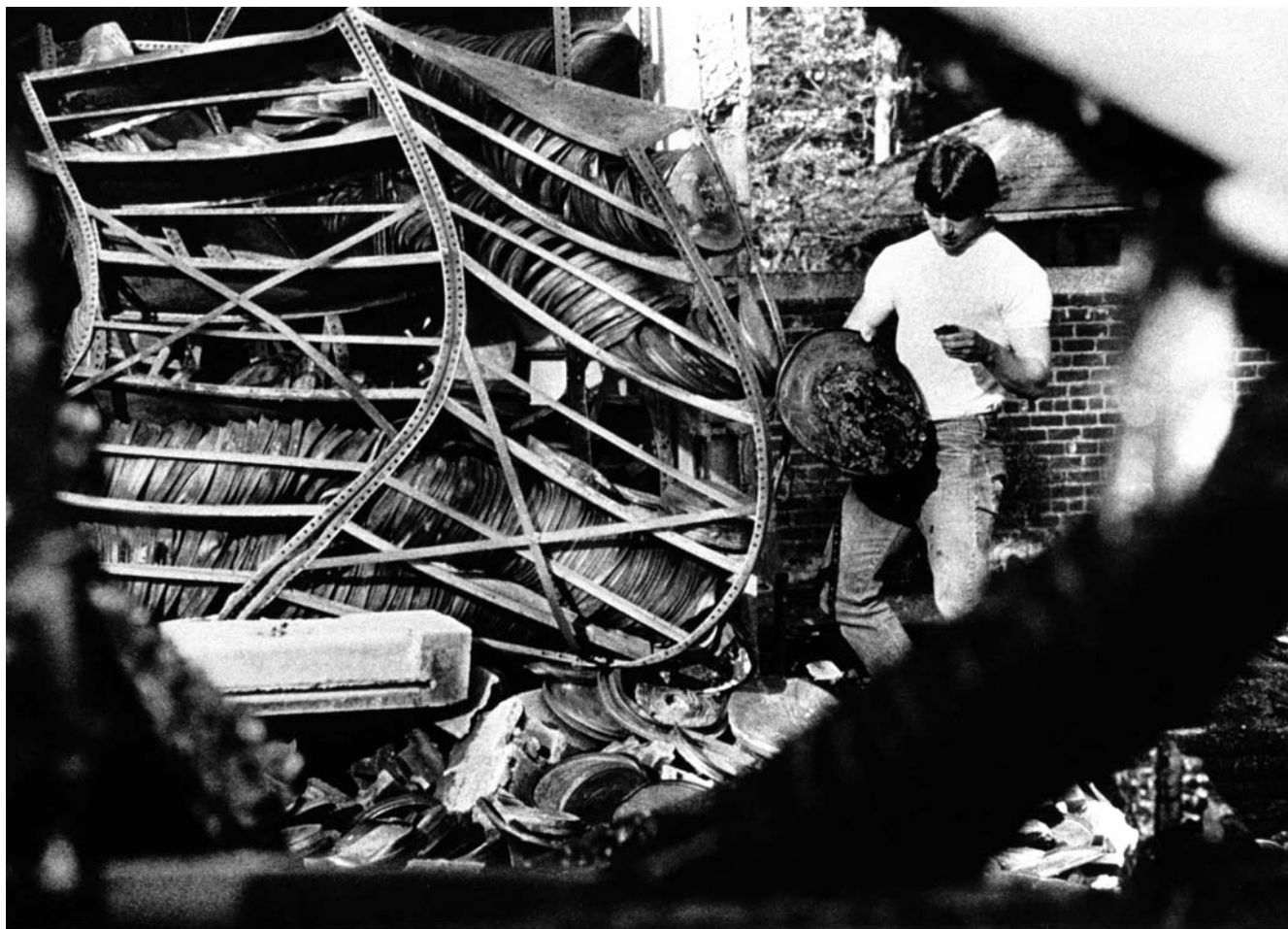
Stored without air conditioning, humidity control, or an alarm system in an abandoned incinerator building on the grounds of the International Museum of Photography at George Eastman House in Rochester, New York, this large store of cellulose nitrate motion picture films ignited on a hot day in May 1978. Original negatives from 329 motion pictures, some of them classics from the early days of the Hollywood motion picture industry, were destroyed in the fire.
