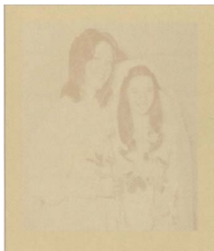
Kodak Ektacolor Plus print after light exposure in an accelerated test equivalent to 250 years of display. (The print was exposed to 21.5 klux glass-filtered fluorescent illumination for 2.7 years [75°F and 60% RH].)
