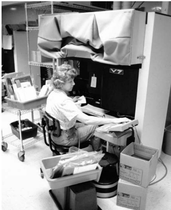
Printer operator Lea Bass printing orders on a Lucht V-7 multi-lens package printer. The daylight printer is loaded with 575-foot rolls of 10-inch Fujicolor paper. H&H also has enlarger stations for prints where custom cropping, dodging, burning, and precise color balance are required.
