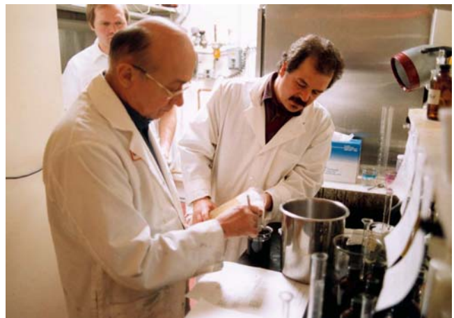
Charles Berger mixing a pigmented-gelatin emulsion for a test coating at Kilborn Photo Products Inc. in Cedar Rapids, Iowa. Working with Berger is John DaSilva, an emulsion chemist who is director of research at Kilborn.
