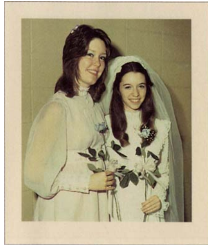
Kodak Ektacolor print after the equivalent of 30 years of display.
