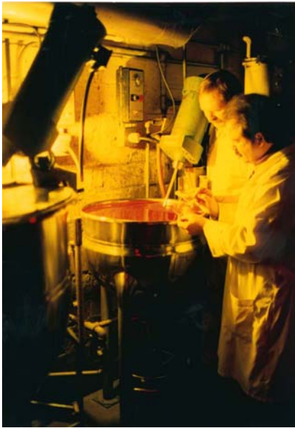
Emulsion technician Steve Hynek and Charles Berger mixing gelatin, magenta pigment, a chromium-free sensitizer, and other emulsion components.
