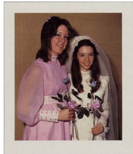
Fujicolor SFA3 color print after the equivalent of 10 years of display.
