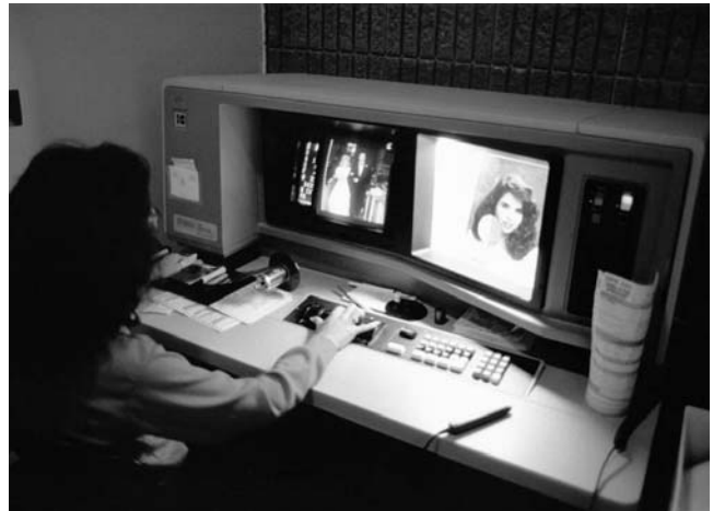
Prior to proofing and printing, each negative is coded and carefully video analyzed with the color balance and density values entered into a networked Digital Equipment Corporation VAX computer system running Kodak Accudata software. When the negative is proofed and later printed, the data are used to control printer filtration and exposure times. Shown here is operator Graciella Marshall with a Kodak PVAC Video Analyzer. H&H also uses Bremson Data Systems CVIS digital video analyzers. Proof prints are individually backprinted with the studio name and date, H&H order number, roll and frame number, and negative density and color filtration values.
